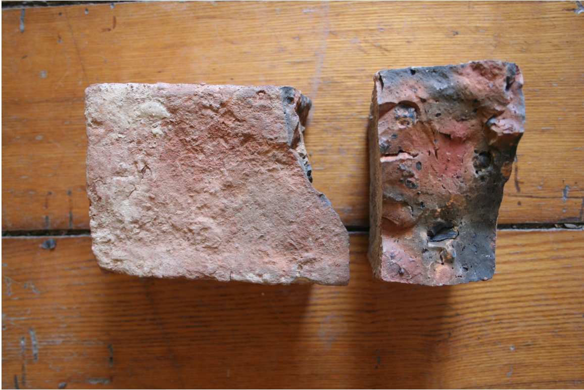
Photo 32. Large moppen bricks used in the construction of the McCutcheon House.
