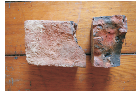
Figure 5. Brick showing dark colored tempering material identified as over-fired brick.
