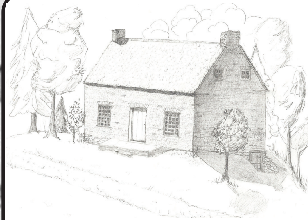
Figure 4. This reconstruction of the front (east) facade of the McCutcheon House is based on archaeological evidence and surviving photographs. Dendrochronology of the structural timbers suggests that the structure was constructed around 1786, the year McCutcheon obtained his lease. Several of the beams dated between 1735-1736, suggesting that some members were recycled from an earlier structure in the vicinity.
